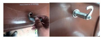
3 Remove nut and washer, insert lock and arm through hole. Replace washers and nut, tighten with shifting spanner or similar.
